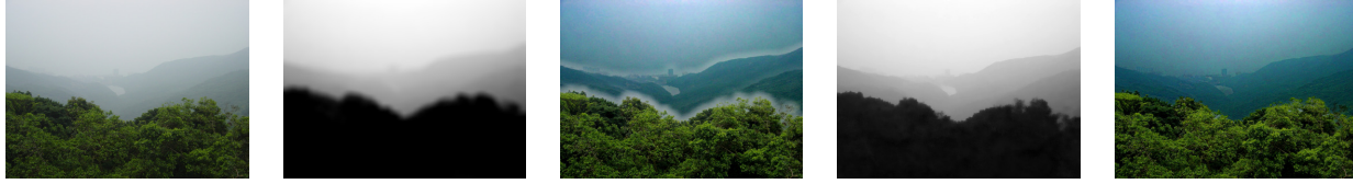
Figure 2. From left to right, the original image, the atmospheric veil V(x, y) and the restoration obtained by enforcing complete smoothness, the atmospheric veil V(x, y) and the restoration obtained by enforcing smoothness most of the time (used parameters in both cases p = 0.95 , s_v = 41 and s_i = 19 ).
