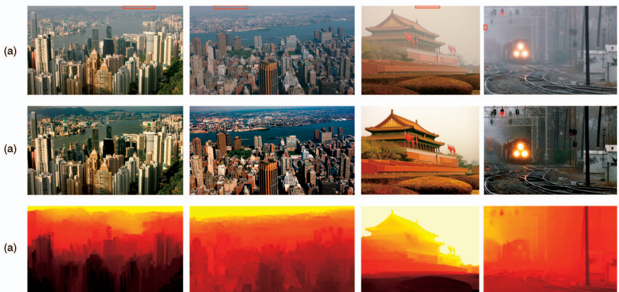
Fig. 12. Haze removal results. (a) Input hazy images. (b) Restored haze-free images. (c) Depth maps. The red rectangles in the top row indicate where our method automatically obtains the atmospheric light.
