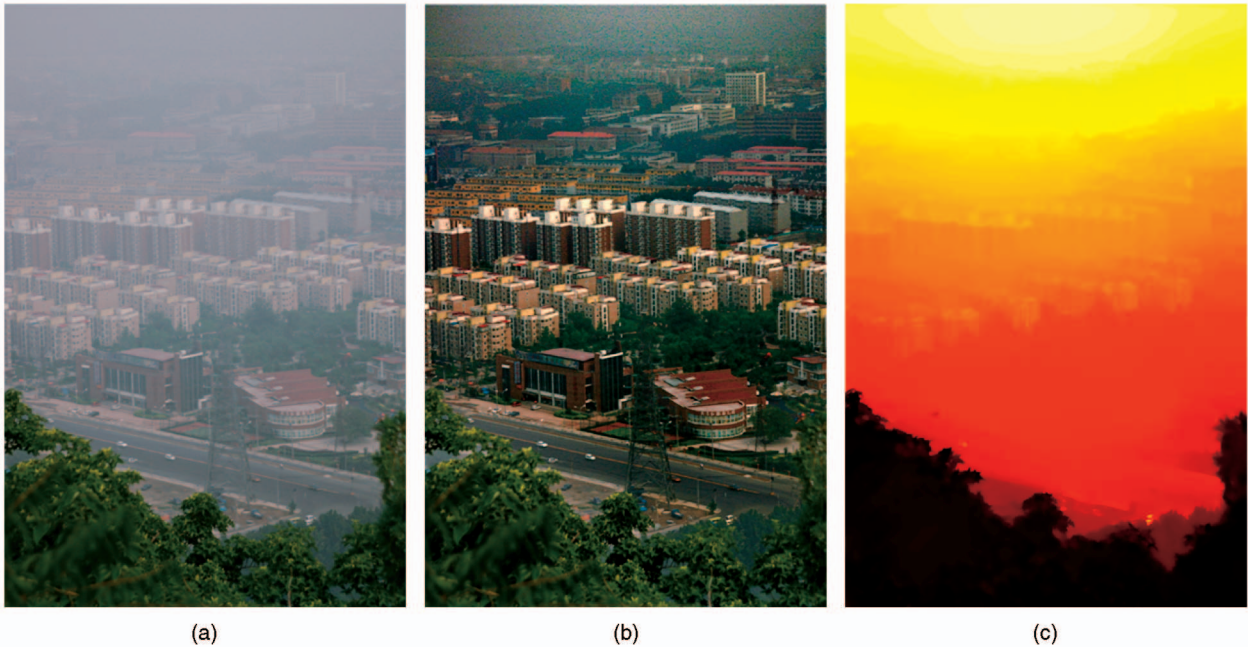
Fig. 1. Haze removal using a single image. (a) Input hazy image. (b) Image after haze removal by our approach. (c) Our recovered depth map.
