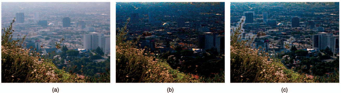
Fig. 10. (a) A 600 \times 400 hazy image and the recovered scene radiance using (b) 3 \times 3 and (c) 15 \times 15 patches, respectively (without soft matting). The recovered scene radiance is oversaturated for a small patch size, while it contains apparent halos for a large patch size.
