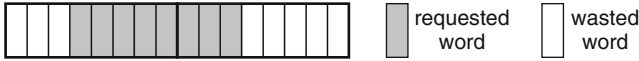
Fig. 3.3 Two bursts of 8 words are required to read or write 8 words that are misaligned
