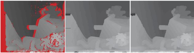
Fig. 3. **Effect of postprocessing.** Postprocessing was applied only in invalidated regions. From left to right: Disparity map with invalidated pixels in red; disparity after scanline-based filling; disparity after applying weighted median filtering for invalid pixels.
