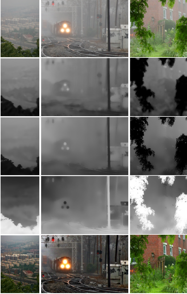
Fig. 7 From top to down: the original images; atmosphere veil obtained through median filtering; atmosphere veil obtained through guided joint bilateral filtering; the transmission map; the dehazed images.
