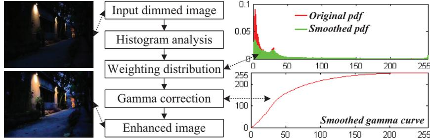
Fig. 1. The flowchart of the proposed image enhancement method.
