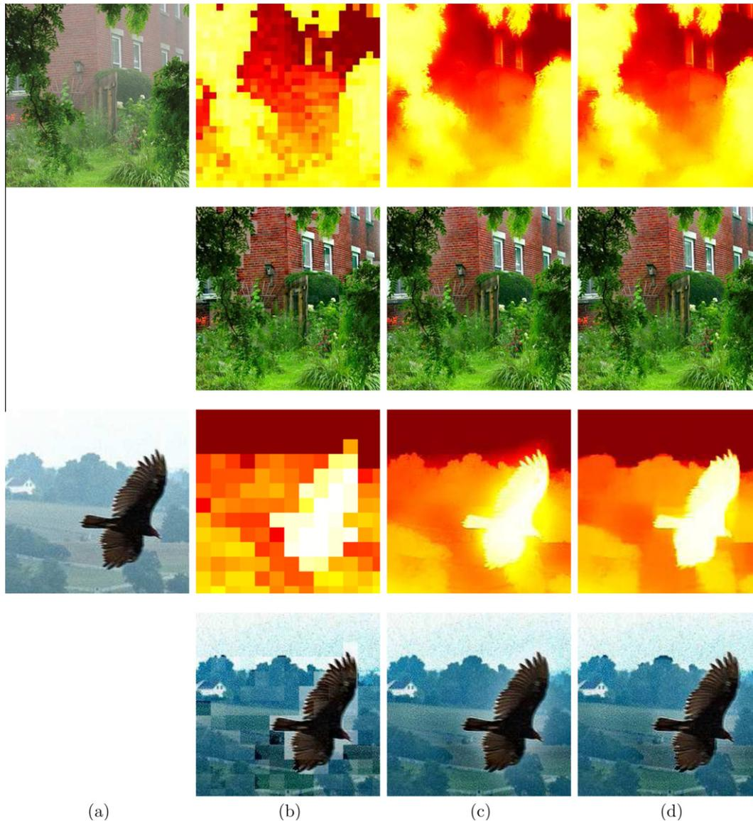
**Fig. 7.** Transmission map refinement: (a) Input hazy images, (b) the block-based transmission maps, and the pixel-based transmission maps using (c) the centered window scheme and (d) the shiftable window scheme. In the transmission maps, yellow and red colors represent near and far scene points, respectively. (For interpretation of the references to color in this figure legend, the reader is referred to the web version of this article.)
